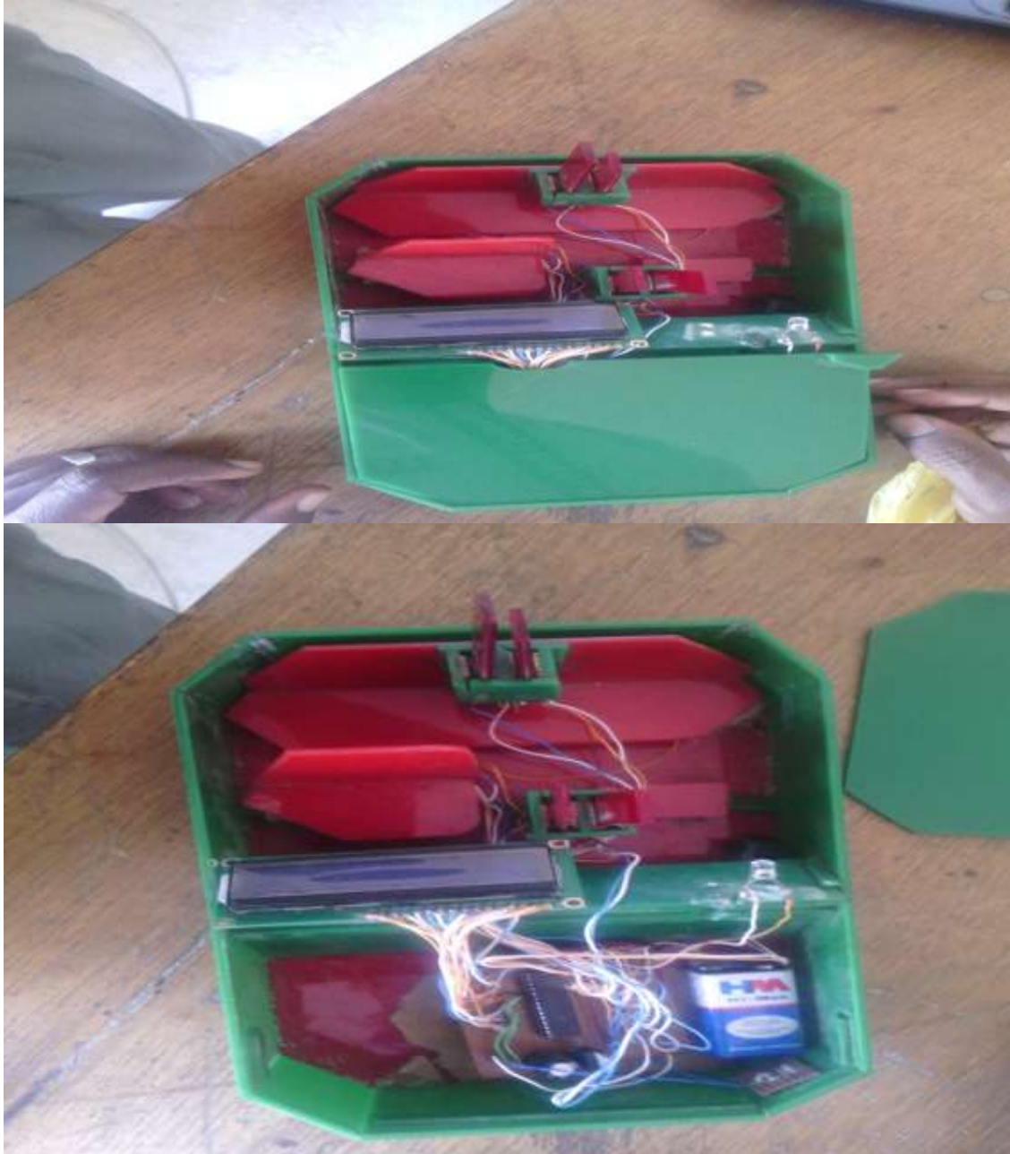
Figure 8: A Prototype of a Car Seat Belt reminder
