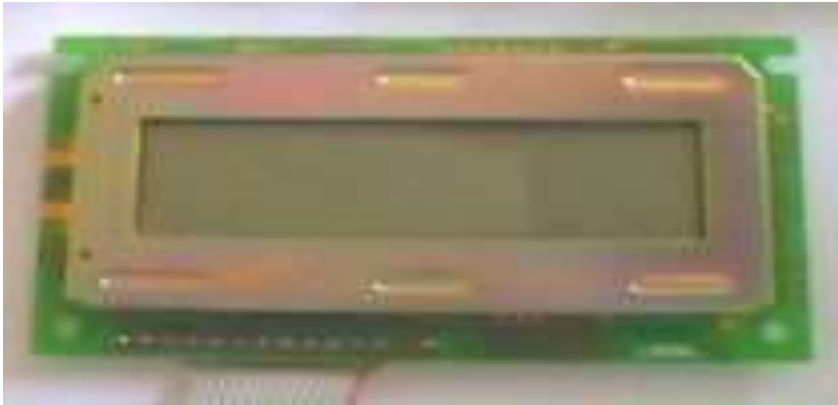
Figure 4: A 16x2 Dot Matrix LCD.
