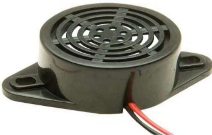
Figure 6: A typical Buzzer.
